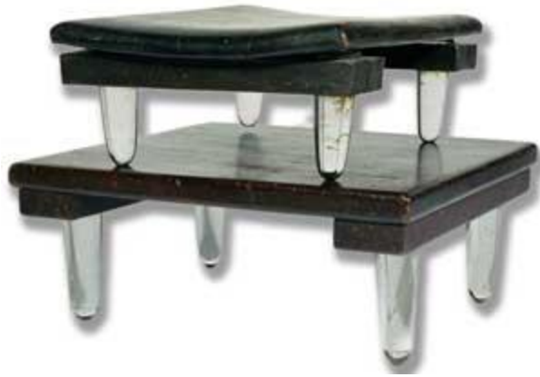
12.10.3 Isolation benches with glass legs
